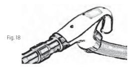
If you use a hose with remote control, you can start and stop the vacuum cleaner using the switch on the handle, Fig. 18.
